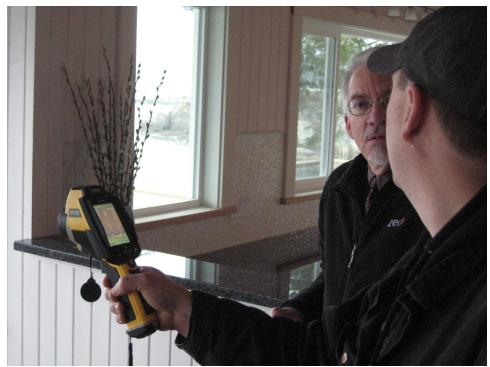
Figure 7: A thermal imaging expert conducts a real-time assessment of heat loss using a hand-held infrared camera with a homeowner. Photo credit: S. Sheppard
