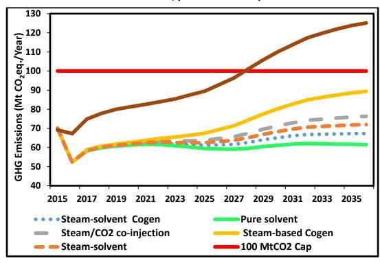
Figure 4.10: GHG Emissions Profile for the Oil Sands Industry and the 100 MtCO<sub>2</sub>/year Emissions Cap
