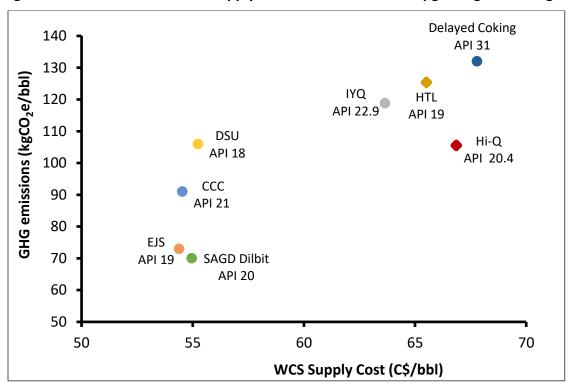
Figure 4.6: GHG Emissions and Supply Cost of Partial and Full Upgrading Technologies
