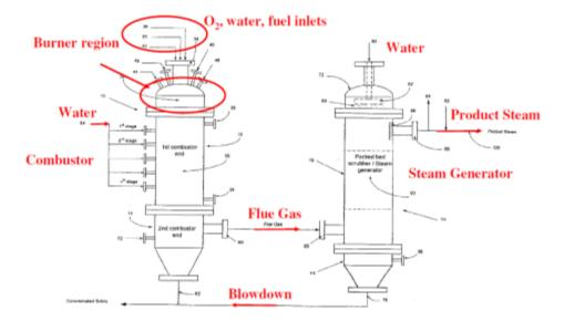
Figure 2.5: DCSG Process and Technology Design
