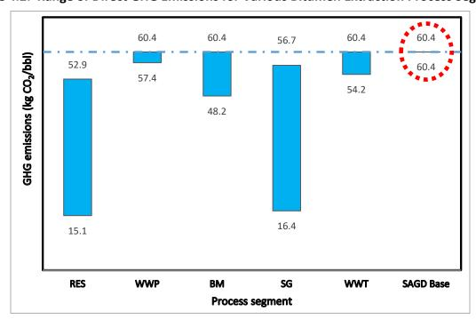
Figure 4.2: Range of Direct GHG Emissions for Various Bitumen Extraction Process Segments
