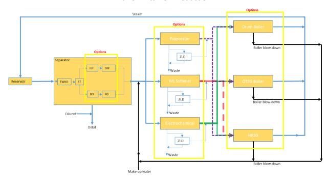
Figure 2.2: Wastewater Treatment and Steam Generation Superstructure for SAGD Bitumen Production
