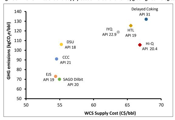
Figure 5.4: GHG Emissions and Supply Cost of Partial and Full Upgrading Technologies
