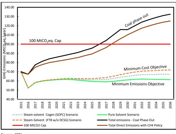
Figure 4.11: GHG Emissions Profile for the Oil Sands Industry and the 100 MtCO<sub>2</sub>/year Emissions Cap with Coal Phase-Out
