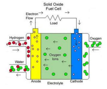
Figure 2.6: Illustrative Diagram of a Solid Oxide Fuel Cell Operation
