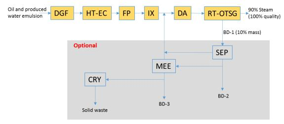
Figure 2.3: Process Flow Diagram of the FTB Process
