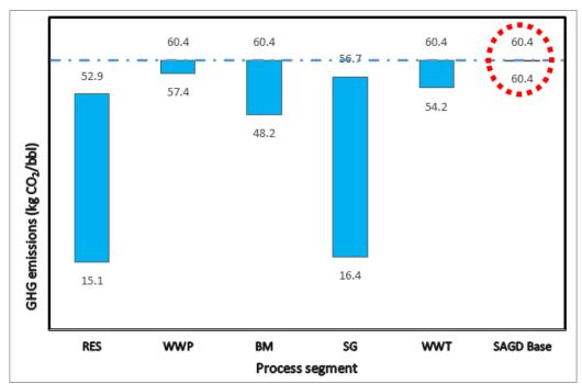
Figure 5.2: Range of Direct GHG Emissions for Various Bitumen Extraction Process Segments
