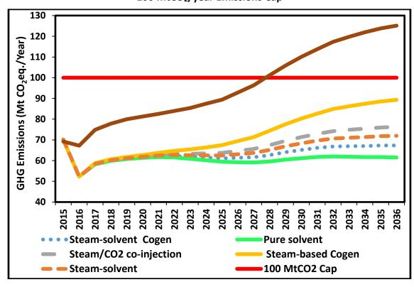
Figure 5.5: GHG Emissions Profile for the Oil Sands Industry and the 100 MtCO<sub>2</sub>/year Emissions Cap
