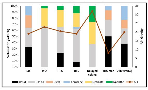
Figure 4.5: Volumetric Yield and API Gravity of Products from Partial and Full Upgrading Technologies
