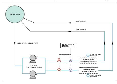
Figure 2.7: Illustrative Diagram of the FC-OSSG Technology
