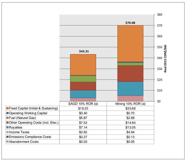
Figure 2.7: Total Field Gate Bitumen/SCO Supply Costs
