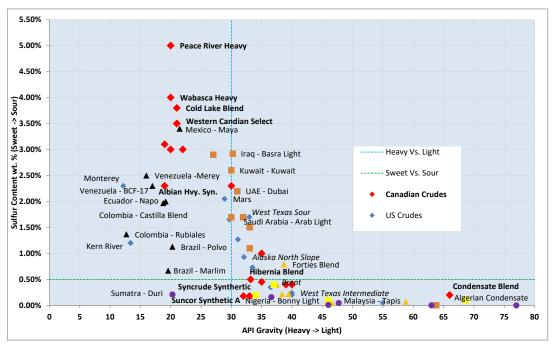
Figure 2.2: Densities and Sulfur Content of Crude Oils
