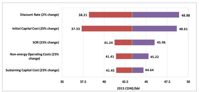
Figure 2.9: Supply Cost Sensitivity – 30 MBPD SAGD Project
