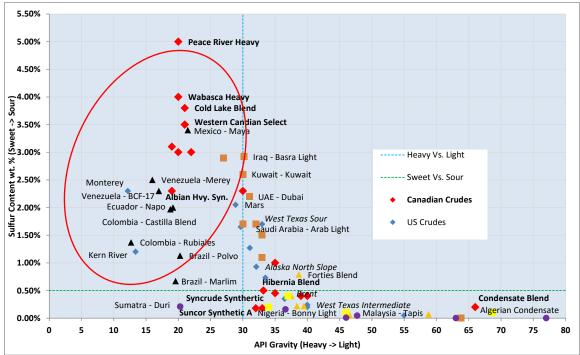
Figure 3.3: Densities and Sulphur Content of Crude Oils
