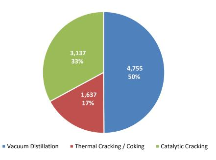
Figure 3.2: 2015 PADD 3 Refining Capacity – Conversion Technologies (thousand barrels per day)
