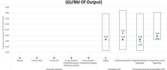
Figure 4.4: Oil Sands Industry Hydrogen Energy Intensity Factors by Project Type (GJ/Bbl Of Output)
