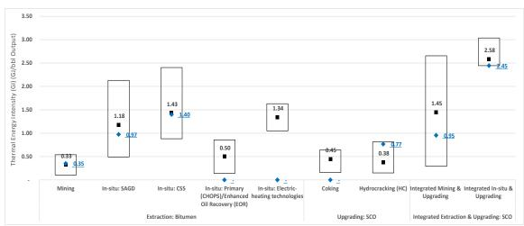
Figure 4.3: Oil Sands Industry Thermal Energy Intensity Factors by Project Type (GJ/Bbl of Output)
