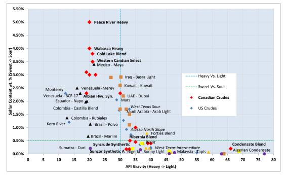
Figure 2.2: Densities and Sulfur Content of Crude Oils
