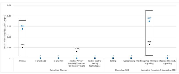
Figure 4.10: Oil Sands Industry Diesel Fuel Intensity Factors by Project Type (bbl diesel/bbl bitumen)
