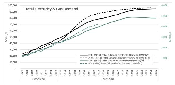
Figure E.8: Oil Sands Industry Electricity (MWh/d) and Gas Demand (MMcf/d)
