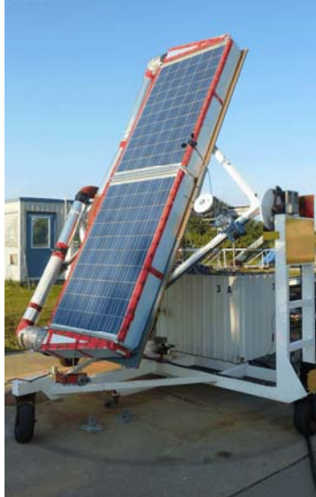
Figure 2 PV/T collector mounted on the outdoor combined PV and thermal testing rig
